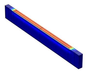
Fig. 2. Uniform SAW displacement amplitude along the aperture of a TC-SAW resonator with properly designed piston mode region. Results are determined from a frequency response COMSOL FEA.
