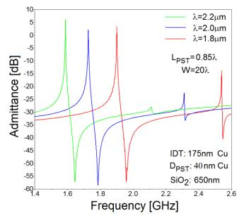
Fig. 5. Measured resonance frequency response of spurious-free TC-SAW resonators with thinner "piston" layer (40 nm) in the border region. All devices have aperture W=20 $\lambda$ , and wavelengths  $\lambda$ =1.8 $\mu$ m  $\lambda$ =2.0 $\mu$ m and  $\lambda$ =2.2 $\mu$ m.
