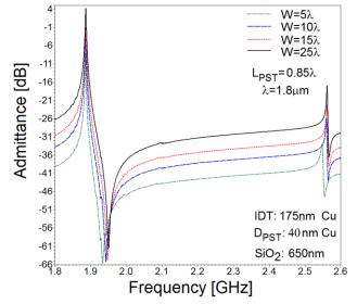
Fig. 4. Measured frequency response of TC-SAW resonators with aperture varying in the range W=5 $\lambda$  to 25 $\lambda$ . Thickness d<sub>PST</sub> and length L<sub>PST</sub> of the loading layer at the border region are kept constant in the vicinity of the optimal quantities for piston shape of the mode.
