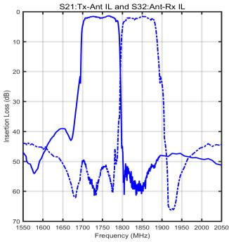
Fig. 8. Measured frequency response a fabricated B3 duplexer employing TC-SAW resonators with piston mode design following the deduced scaling rules.
