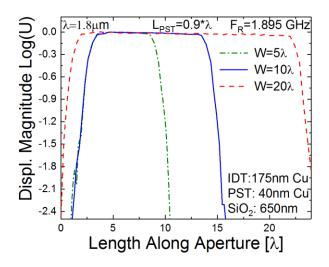
Fig. 3. Simulated distribution of the normalized total displacement magnitude along the aperture of TC-SAW resonators with varying apertures. Resonators with pitch p=0.9 ( $\lambda$ =2p=1.8µm) were simulated while varying the aperture W. The spurious control was seen to be insensive to this dimension.
