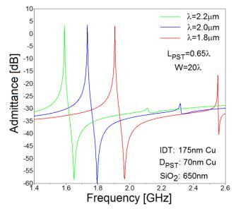
Fig. 6. Measured resonance frequency response of spurious-free TC-SAW resonators with thicker "piston" layer (70 nm) in the border region. All devices have aperture W=20 $\lambda$ , and wavelengths  $\lambda$ =1.8 $\mu$ m  $\lambda$ =2.0 $\mu$ m and  $\lambda$ =2.2 $\mu$ m.
