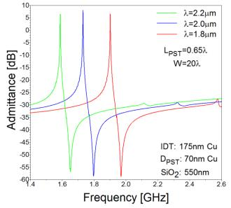
Fig. 7. Measured frequency response of TC-SAW resonators with aperture W=20 $\lambda$ , and wavelengths  $\lambda$ =1.8 $\mu$ m  $\lambda$ =2.0 $\mu$ m and  $\lambda$ =2.2 $\mu$ m. The thickness d<sub>PST</sub> and length L<sub>PST</sub> of the loading layer at the border region are kept constant in the vicinity of the optimal quantities for the piston mode.
