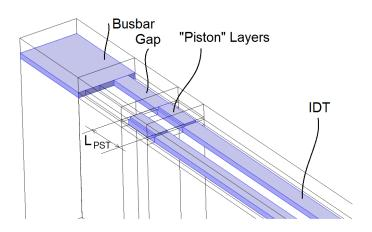
Fig. 1. Close view of a 3D COMSOL model in the vicinity of the border region. The additional layer of piston mass has length is  $L_{PST}$  and thickness  $d_{PST}$ .
