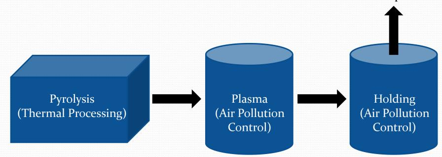
The CoronaLux System order of operations ensures that the downstream air pollution control systems are fully operational before any medical waste is processed.
