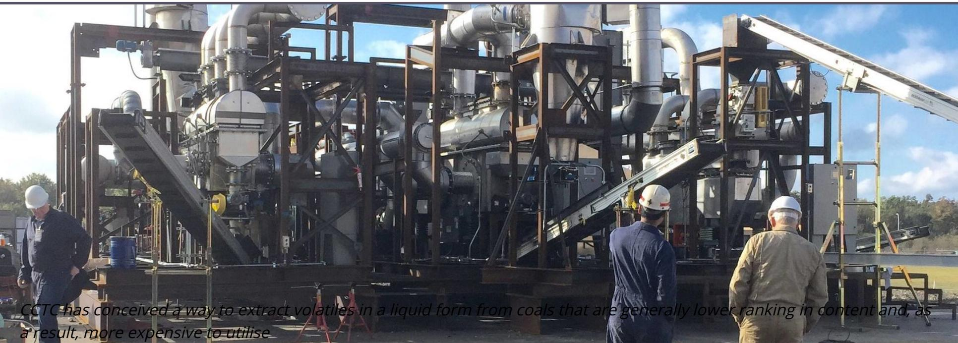
*CCTC has conceived a way to extract volatiles in a liquid form from coals that are generally lower ranking in content and, as a result, more expensive to utilise*
