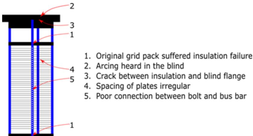
*Diagram 1: Conceptual Drawing of Current Stack*
