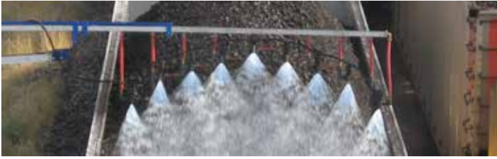
Figure 1. Coal sprayed with water and chemicals to reduce coal dust loss during transportation.
