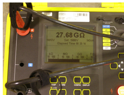
Display of an Ohmmeter, a scientific instrument used to measure electrical resistance, showing a reading of 27.68 giga-Ohms during testing of retrofitted AOT unit.
