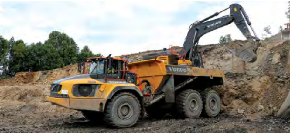
At Point Lick Energy's Camel Creek site, three Volvo A60H 60-ton articulated haulers manage about 98% availability over a six-month period. (Photo: Volvo Construction)
