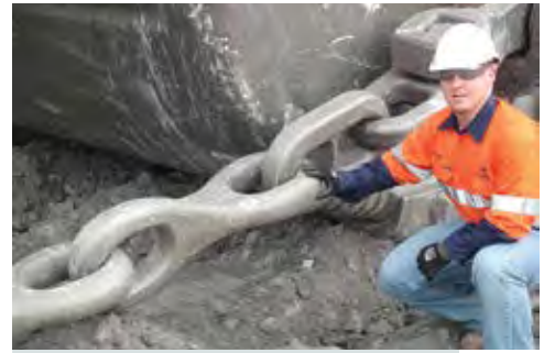
Columbia Steel's TwistLink weighs roughly 22% less than standard chain equivalent. (Photo: Columbia Steel)
