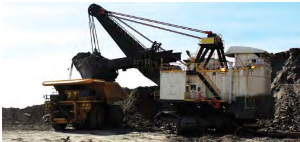
FLANDERS’s Freedom shovel upgrades employ a detailed cycle decomposition algorithm that helps determine when certain functionalities should be used, the company reports. (Photo: FLANDERS)
