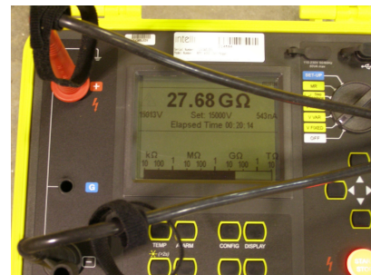
Display of an Ohmmeter, a scientific instrument used to measure electrical resistance, showing a reading of 27.68 giga-Ohms during testing of retrofitted AOT unit.
