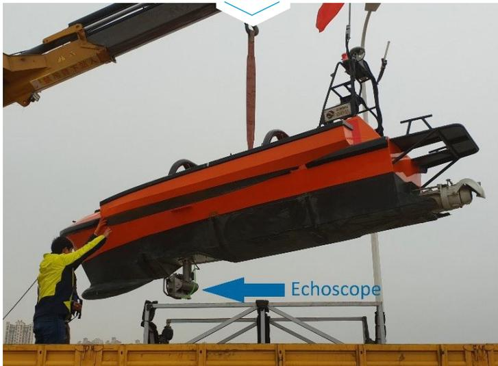
Coda Octopus has recently partnered with AVIC IET, an offshore wind contractor in China, to integrate the Echoscope4G® Surface real-time 3D sonar on a state-of-the-art Autonomous Surface Vehicle (ASV).
