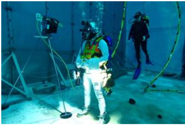
Diver, center, with Gen 2 DAVD system mounted on Kirby Morgan KM97 helmet being tracked at NASA's Neutral Buoyancy Laboratory; Echoscope® C500 Inspector system, left.
